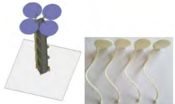
The antenna's quadrifilar helix design and components created using 3D printing
